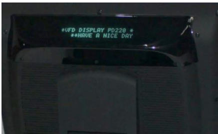
LCD or VFD Customer Display 2 lines * 20 Characters
